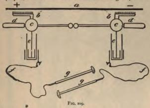
resents the interrupted primary circuit of a Holtz machine without condensers, a, standing for the rotating plates, bb, collecting combs, cc, prime conductors, dd, discharging rods, f, f, conducting cords, gi, sponge or other electrodes.
